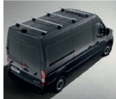
Transverse roof bars
