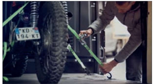
TIE-DOWN HOOKS incorporated to ballast the load.
