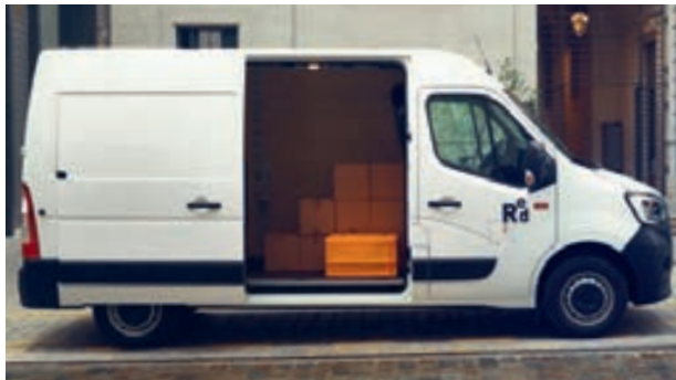
SIDE DOOR WIDTH UP TO 1,270 MM for loading europallets.
