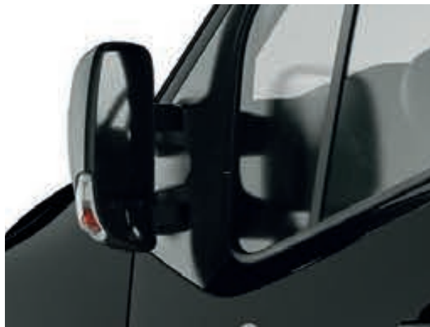
2 WIDE ANGLE MIRRORS electrically adjustable with integrated indicators.
