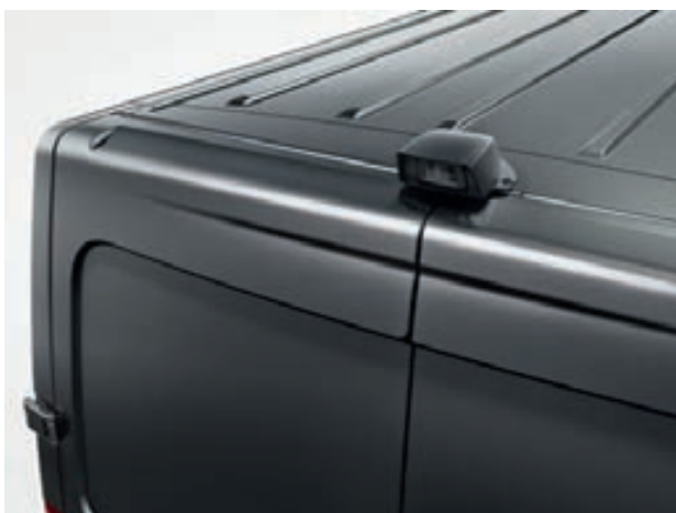
3 CONSTANT REARVIEW (OPTION) via a camera on the rear of the roof acting as a rearview mirror while driving.
