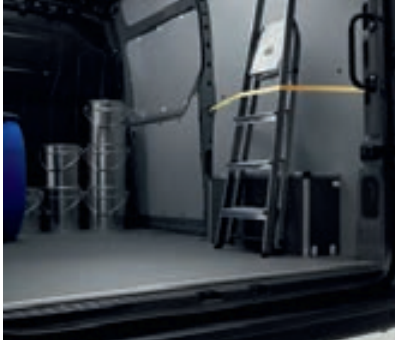
6 mm polypropylene side walls and non-slip floor
